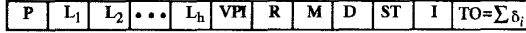
Figure 4: The SETUP packet with its fields. The first field P is the parity bit. The path of the SETUP packet is specified as a sequence of link identifiers L_1, L_2, \dots, L_h , corresponding to the links that the packet must traverse. The virtual path identifier field VPI, is a 12 bit field that specifies the virtual path number of each session for a particular hop along its path. The requested rate field R is the rate required by the session. The minimum rate field M is the minimum rate with which the session will be satisfied; in general, we may have M \neq R . The D field is used by the intermediate nodes to decide whether the session can be accepted or not. If the intermediate node has sufficient residual capacity available starting at a time earlier than the maximum delay, the session is accepted, otherwise it is rejected.
