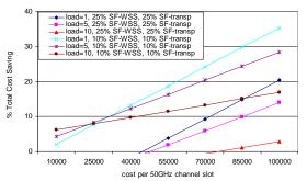
Fig 3. Percentage of additional cost of the SF transponder over the cost of the 100 Gpbs transponder as a function of the cost of the 50 GHz slot, for different SF-WSS extra cost percentages and for load=5.
