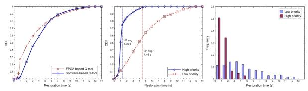
Fig. 3. Performance evaluation: lightpath restoration time CDF with and without FPGA acceleration (left); lightpath restoration time CDF for high and low priority traffic classes (center); lightpath restoration time frequency for high and low priority traffic classes (right).
