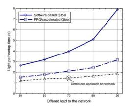
Fig. 3. Average light-path setup time vs. offered load (Erlang).
