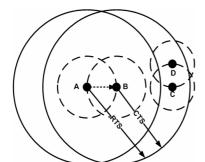
Figure 1 - The IEEE 802.11 approach. Solid lines represent the receiving areas of the RTS and CTS frames when the maximum transmission power is used, while dashed lines represent the transmission ranges of the nodes when the minimum required power for coherent reception is used.
