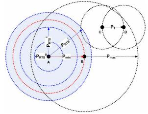
Figure 2 – Proposed power control scheme. The transmission between nodes C and D can take place, even though both nodes have received a CTS frame from node B.
