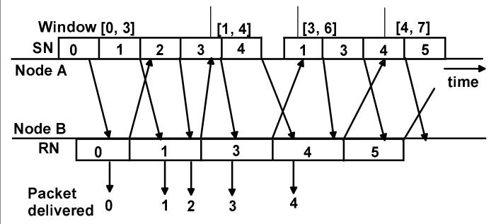
Long frames in the feedback direction slow down ACKs and may cause a transmitter with short frames to wait or (if time-out expires) to go back.
