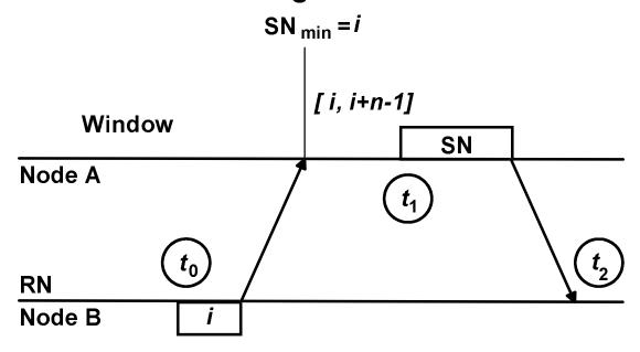
Let  $rn = RN \mod m$   $sn_{min} = SN_{min} \mod m$  $sn = SN \mod m$
