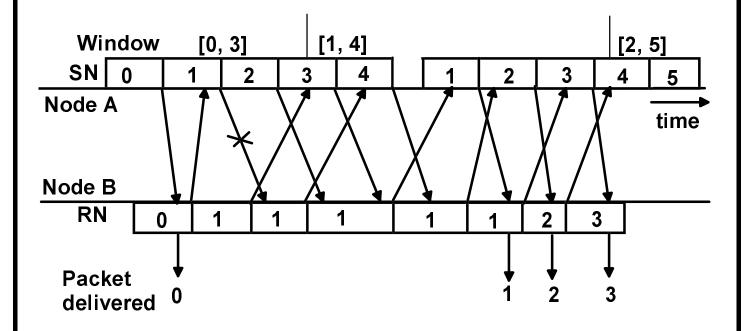
Example 3: (retransmissions due to feedback errors for go back n)
