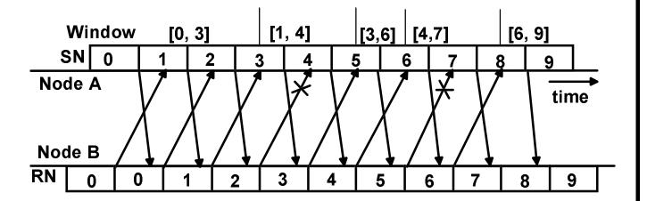
**Example 2**: (retransmissions because of errors for go back 4)
