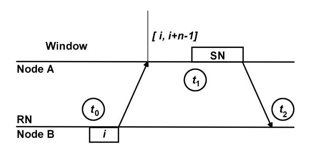
$$SN_{\min}(t_1) \leq SN \leq SN_{\min}(t_1) + n - 1$$
