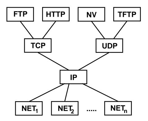
FTP = File Transfer Protocol HTTP = Hyper-Text Transport Protocol NV = Network Video TFTP = Trivial File transport Protocol TCP = Transport Control Protocol UDP = User Datagram Protocol IP = Internet Protocol
