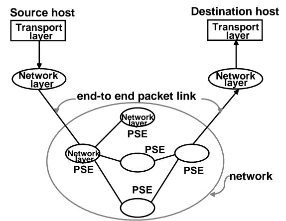
Packets may be delivered to the higher layers in the correct order (virtual circuit service) or out of order (datagram service).
