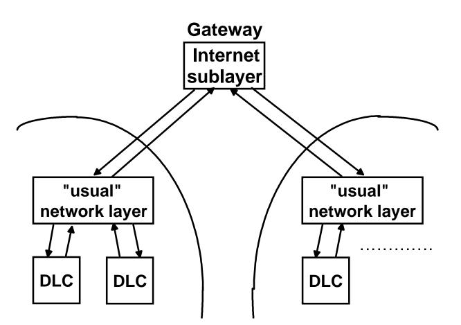
**Function:** routing and flow control between networks, conversion of packet format etc.
