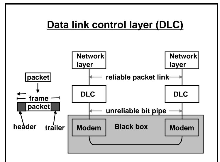
**Function:** framing, error control, retransmissions.
