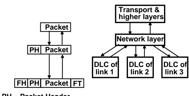
PH = Packet Header FH = Flame Header FT = Frame Trailer
