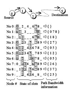
Fig. 4. An example for bandwidth calculation and reservation. The number of data slots is 10. "\_" means a reserved slot by the other connections. Bandwidth requirement is two data slots per frame.
