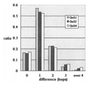
Fig. 16. Difference between the number of hops each packet took to reach its destination and the optimal number of hops required.
