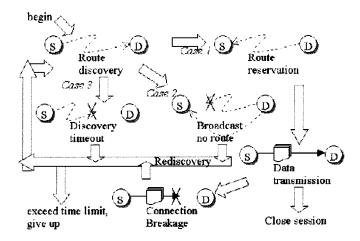
Fig. 6. Overview of the on-demand routing algorithm.
