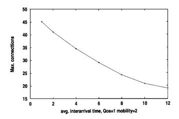
Fig. 12. The maximal number of connections for  $QoS_1$  traffic.
