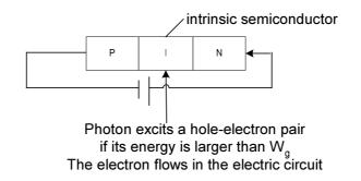
Material of PIN diode is the same with that of LED or LD
