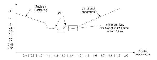
low loss window of width 100nm at  $\lambda$ =1.33 $\mu$ m
